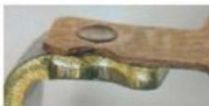
導電端子焊接 Terminal Welding
